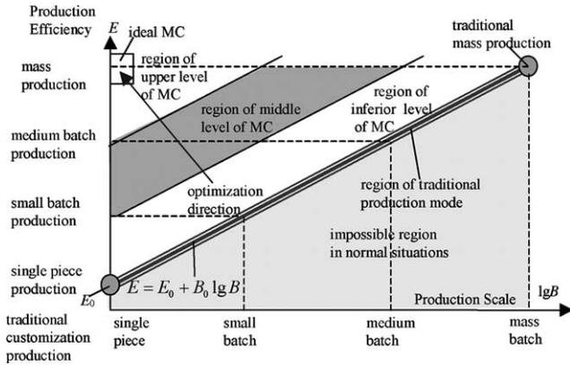
Fig. 1. The efficiency optimization model for MC.
