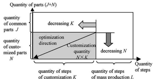
Fig. 2. An optimization model for minimal customization quantity.
