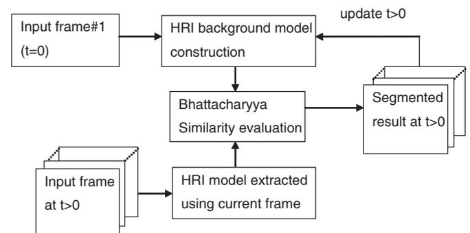
Fig. 1. Block diagram of the proposed approach.
