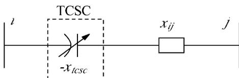
Fig. 2. Steady-state equivalent circuit of TCSC.
