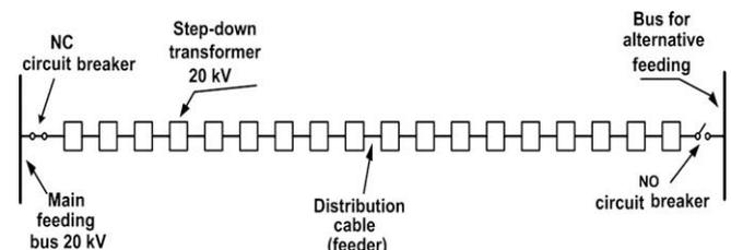
Fig. 2. Typical layout of urban distribution feeder.
