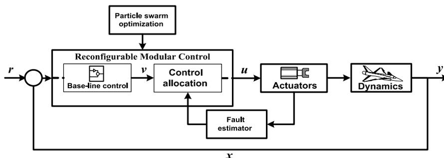
Fig. 1 Structure of optimized reconfigurable flight control system
