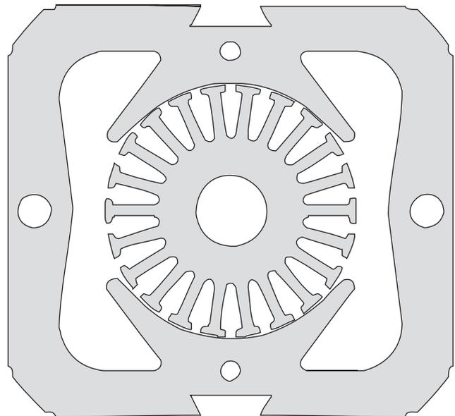
Fig. 2. Stator and rotor laminations of a UM.
