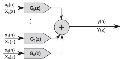
Fig. 2. The Z-transform artificial neuron after simplification.
