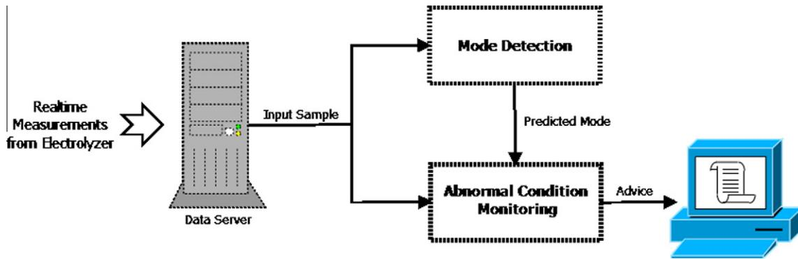
Fig. 1. Block diagram of the Advisory System, showing its main modules.
