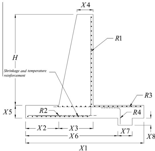
Fig. 1. Design variables for general retaining wall.
