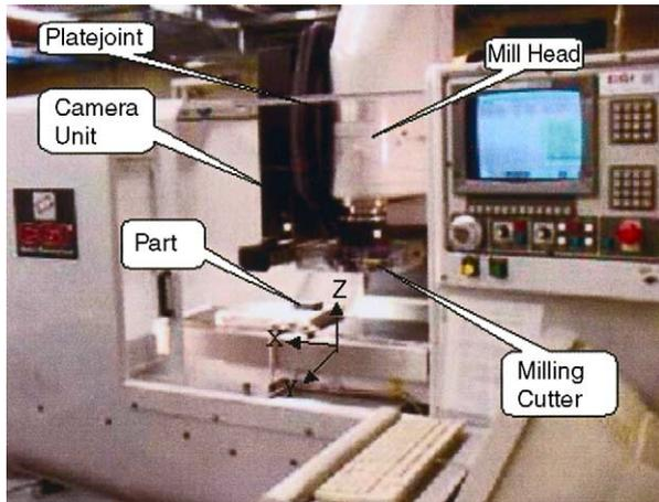
Fig. 1. Machine set up and machine co-ordinates.
