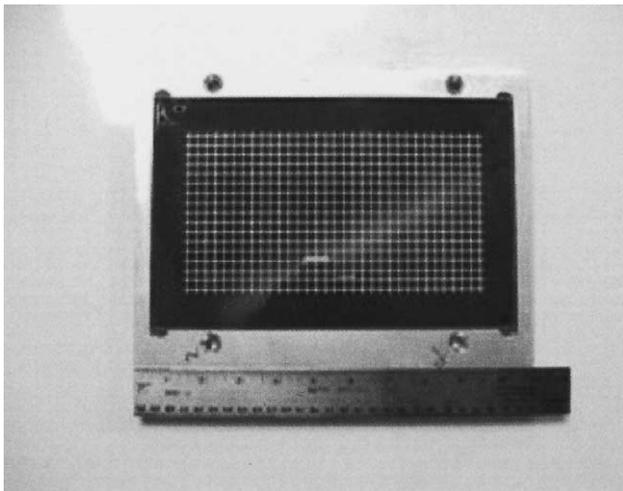
Fig. 2. Optical grid.
