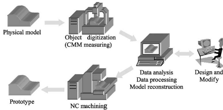
Fig. 1. Working processes of RE.
