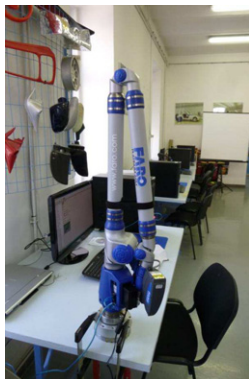
Fig. 1 FARO Platinum Arm with Laser ScanArm in Automotive production section Lab
