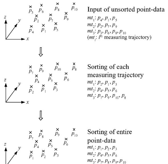
Fig. 1. Basic concept of sorting of 3D point data.
