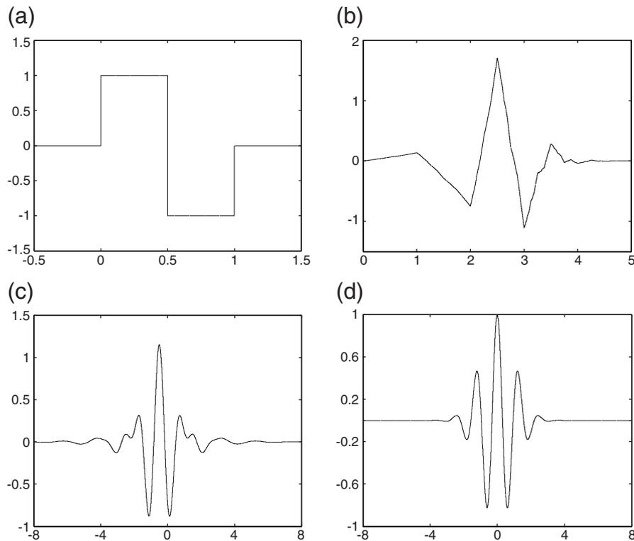
Fig. 1. Some wavelet examples: (a) Haar wavelet, (b) Daubechies wavelet (of order 3), (c) Meyer wavelet, and (d) Morlet wavelet.
