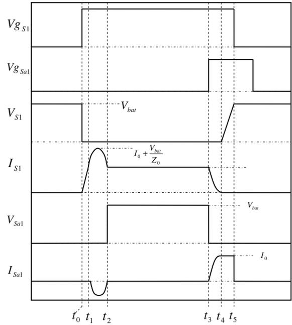
Fig. 2. Converter theoretical waveforms in buck mode.
