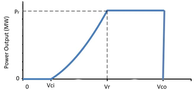
Fig. 1. Power curve of a wind turbine.
