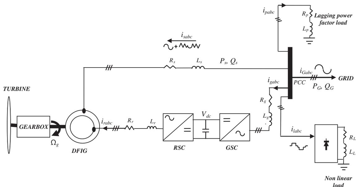
Fig. 1. Synoptic scheme of the studied WECS.
