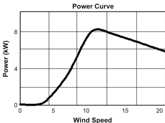
Fig. 1. Wind turbine power versus wind speed characteristic [7].
