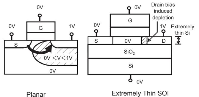
Fig. 3. Planar and extremely thin SOI MOSFETs.
