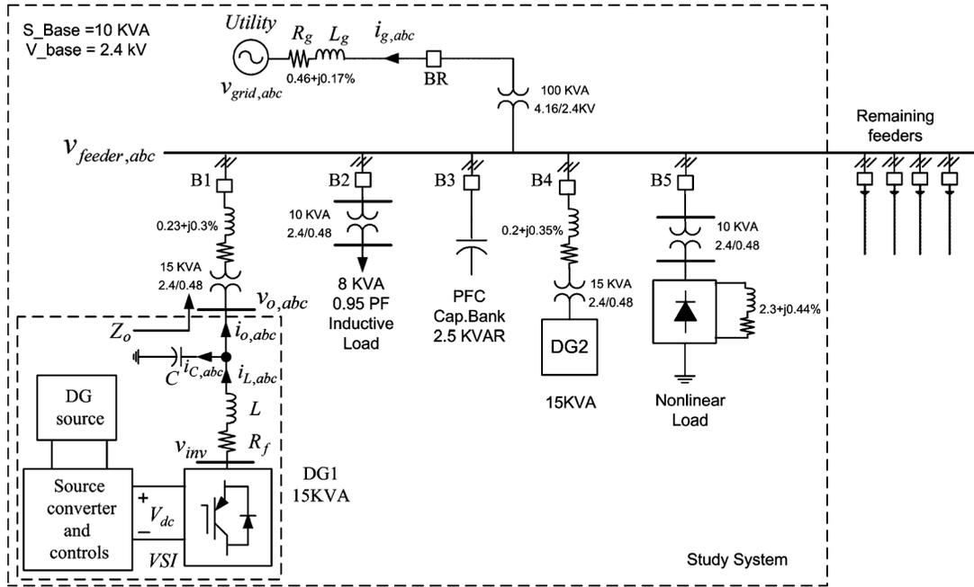
Fig. 1. Single line diagram of the micro-grid study system.
