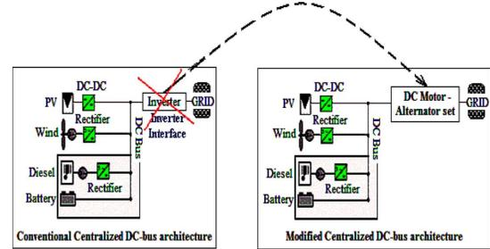
Fig. 3. Comparison of conventional and retrofitted HPS.
