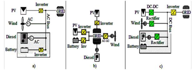
Fig. 2. Different architectures of grid connected HPS.
