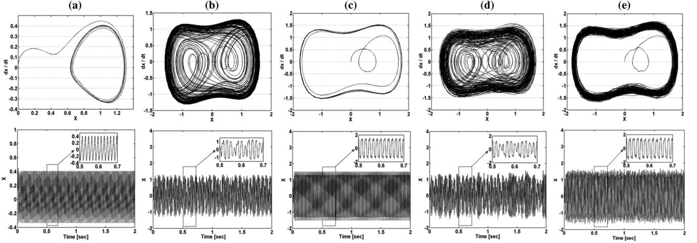
Fig. 1. Duffing oscillator in the phase plane and  $x - t$  diagram. (a) Small periodic motion. (b) Chaotic motion. (c) Great periodic motion. (d) Chaotic motion additional Gaussian noise. (e) Great periodic motion-added Gaussian noise.
