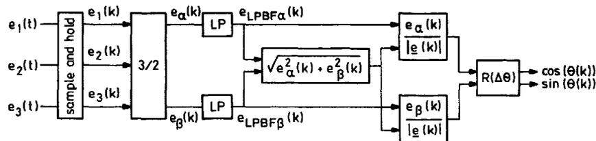
Fig. 2 Diagram of LP-TAD
