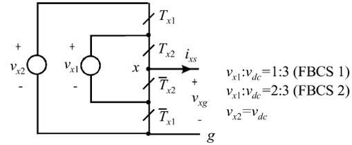
Fig. 2. Two-cell four-level floating voltage source inverter topology.
