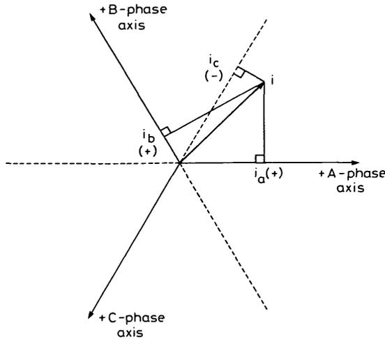
Fig. 1 Vector representation of instantaneous three-phase variables
