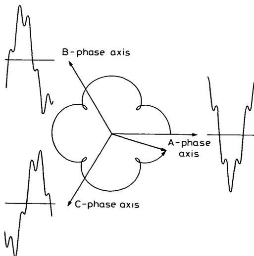
Fig. 2 Example of vector trajectory: 25% fifth harmonic
