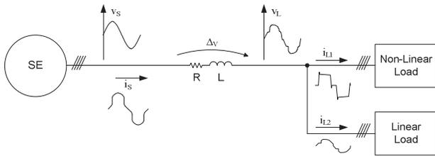
Figure 1. Harmonic distortion propagation.
