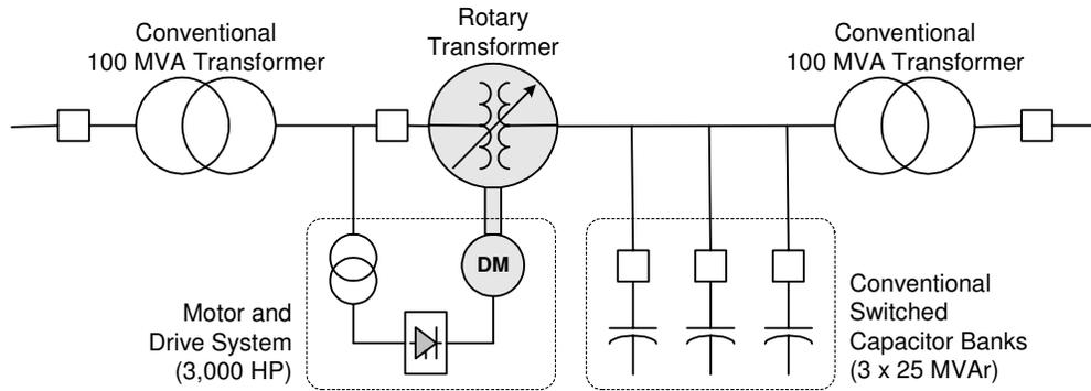
Figure 2. One-line diagram of Langlois VFT.
