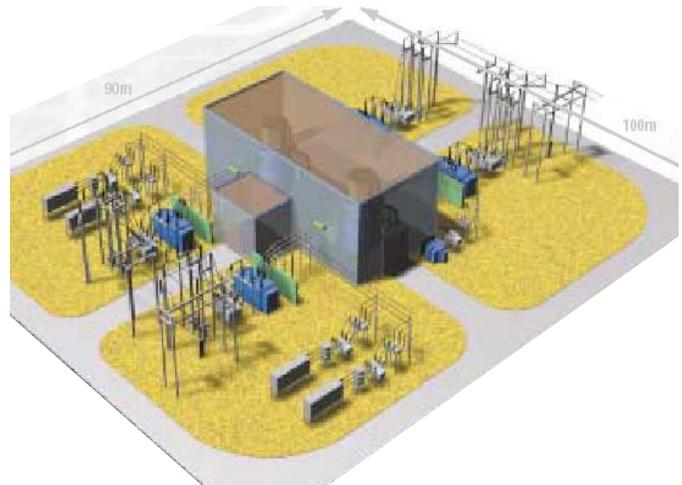
Figure 3. Physical layout of a 200 MW VFT station with two units.
