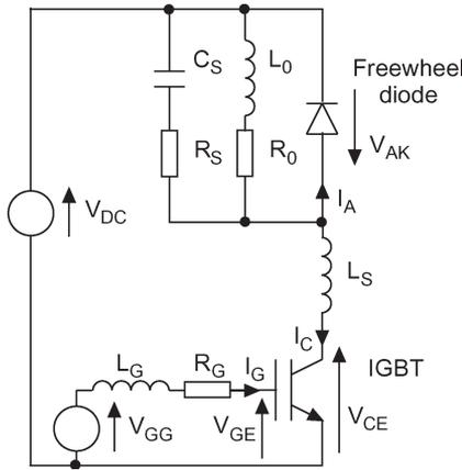
Fig. 2. Single chopper cell ( $R_0, L_0$ : load;  $R_S, C_S$ : snubber;  $L_S$ : stray inductance;  $L_G, R_G$ : gate inductance; and  $R_G$ : gate resistance).
