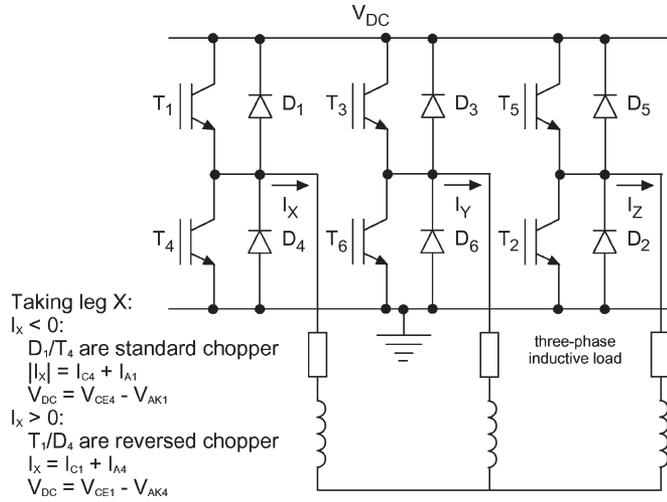
Fig. 1. Reduction of full bridge taking phase  $X$  as an example.
