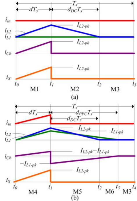
Fig. 3. Key waveforms of the proposed S4 converter: (a) in region I and (b) in region II.
