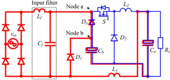
Fig. 1. Proposed transformerless S4 converter.
