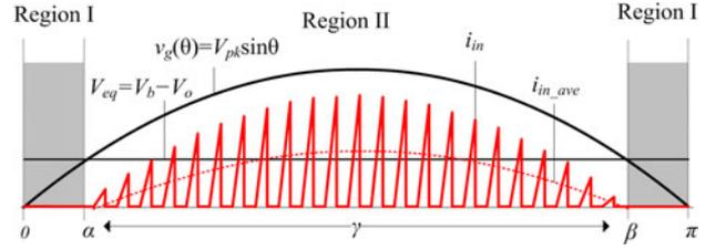
Fig. 2. Two working regions of the proposed S4 converter.
