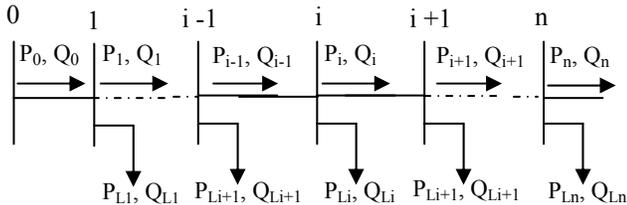
Fig. 1 Single-line diagram of a main feeder
