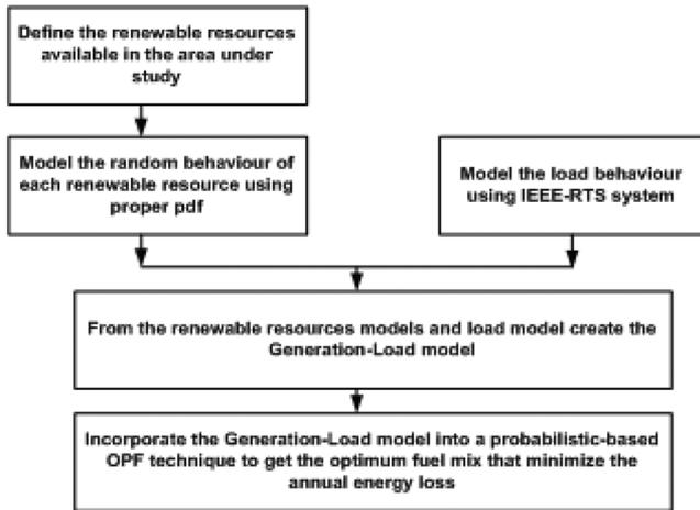
Fig. 1. Block diagram of the proposed work.
