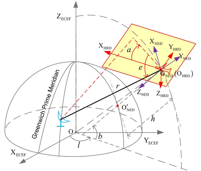
Fig. 1. Coordinate systems involved for airborne platforms.
