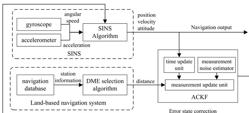
Fig. 1. Structure diagram of inertial and land-based integrated navigation system.
