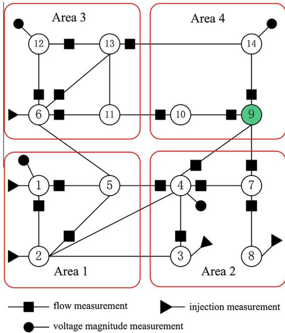
**Fig. 1.** The IEEE 14-bus system divided into four areas. PMU bus 9 shown as a green circle. (For interpretation of the references to colour in this figure legend, the reader is referred to the web version of this article.)
