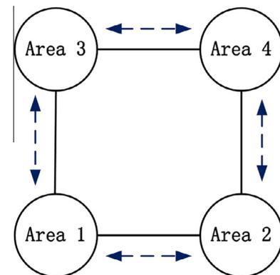
**Fig. 2.** The communication graph of IEEE 14-bus system.
