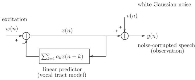
Fig. 1. Block diagram showing the speech production model (linear predictor) and white Gaussian noise that is added to the speech.
