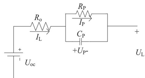
Fig. 1. Schematic of the *Thevenin* battery model.
