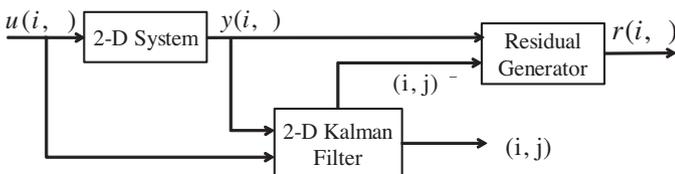
Fig. 1. Structure of a 2-D Kalman filter based residual generator.
