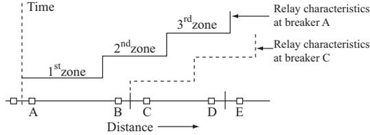
Figure1: Distance relay protection
