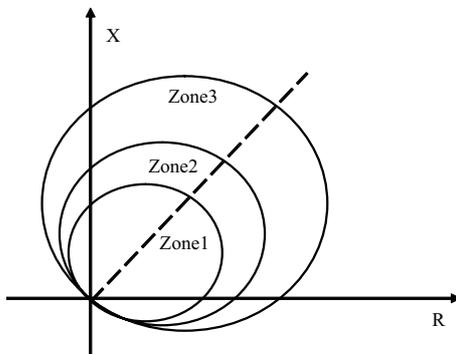
Figure2: Operating Characteristics of mho type distance relay
