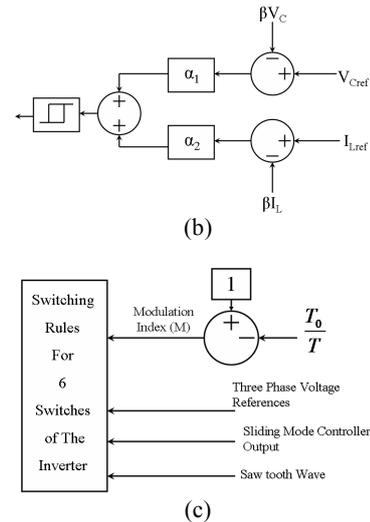
Fig.3. Schematic diagram of SM controlled ZSI. (a) z source and controller. (b) hysteresis sliding mode controller for output network impedance voltage. (c) Controller of inverter switching
