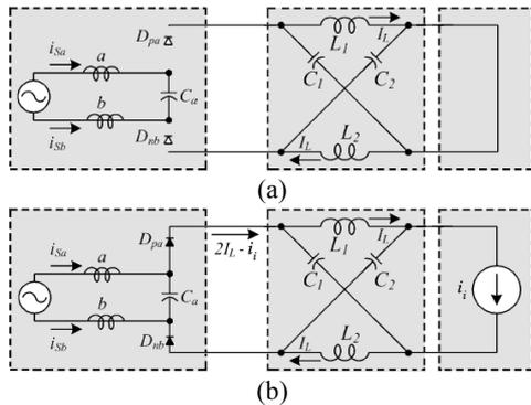
Fig. 2. Equivalent circuits of ZSI. (a) shoot-through mode. (b) Non-shoot-through mode
