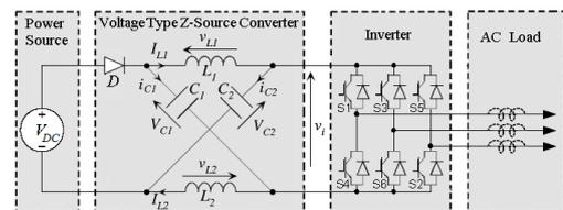
Fig.1 Schematic configuration of a z-source inverter
