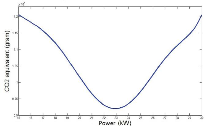
Fig. 4: CO<sub>2</sub> equivalent emissions obtained for a 30kW turbine
