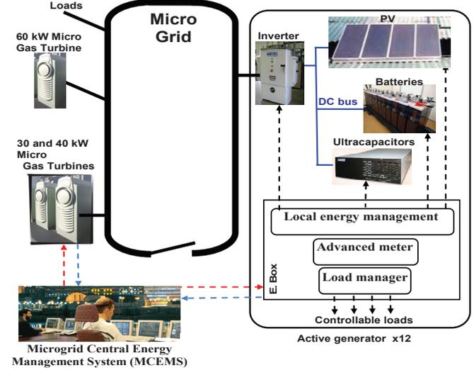
Fig. 3: Microgrid including 12 active generators, 3 gas turbines and a central energy management
