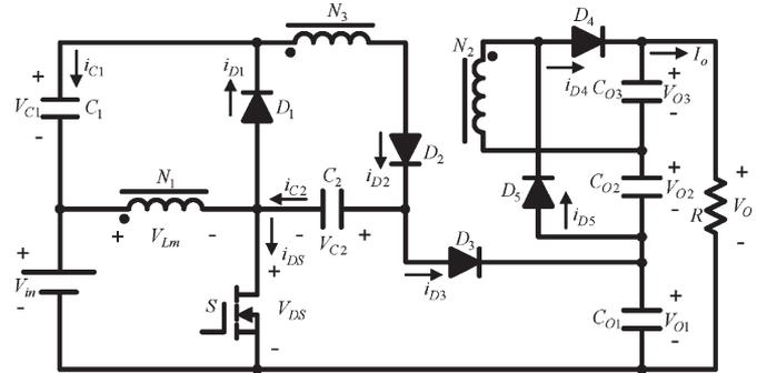
Fig. 2. Circuit configuration of the proposed converter.
