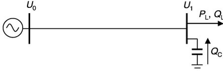
Fig. 1. One-line diagram of a simple two-bus system.
