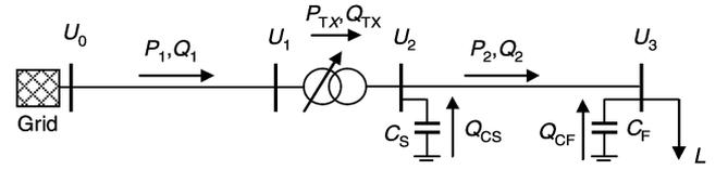
Fig. 2. One-line diagram to illustrate the voltage and reactive power control.
