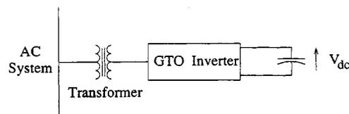
Fig. 1. Connection of a StatCom to a bus.
