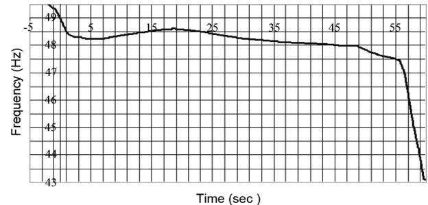
Fig. 1. Falling frequency during blackout on December 14, 2007 from DFDR records.
