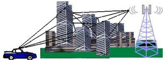
Figure 1. Multipath fading problem in wireless communication at vehicular speeds.
