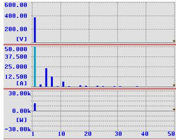
Figure 3. A- phase harmonic voltage, current and power histogram
