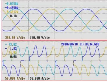
Figure 2. Waveform of three-phase voltage and current
