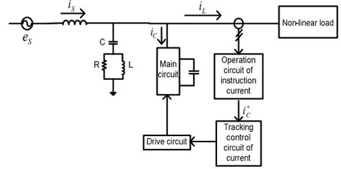
Figure 4. System configuration of Active Power Filter
