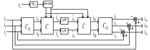
Figure 5. Principle diagram of  $i_p-i_q$  detecting method
