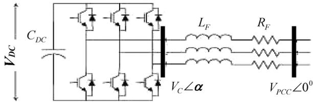
Fig. 1. Schematic diagram of DSTATCOM.
