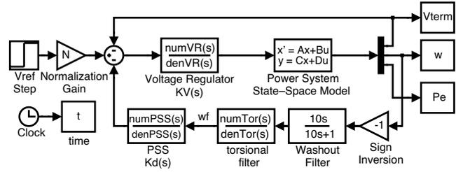
Fig. 2. Control structure of the single-machine infinite-bus system.
