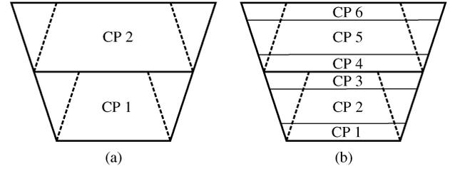
Fig. 3. Sectioning of the 3-D in geometry into the different computation planes (CP): (a) used in the optimization, and (b) used in simulations.
