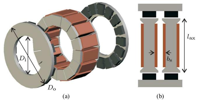
Fig. 1. Topology of the PMSM showing the parameters to optimize. (a) Overview. (b) Detailed view of a tooth pitch.
