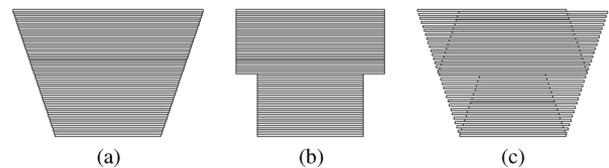
Fig. 2. Different stack configurations of the laminations: (a) ideal full overlap, (b) full overlap with two different lamination types, and (c) alternated with two different lamination types resulting in zones with only partial overlap.
