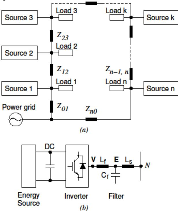
Fig. 1. Microgrid with distributed sources and loads
